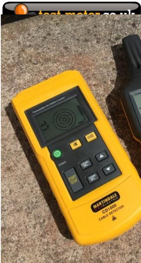
The Martindale transmitter is the more complex of the two, given its greater feature set. It has separate buttons to select power on/off, mute, torch feature, start/stop transmitting, select level, select code and adjust values up and down.
