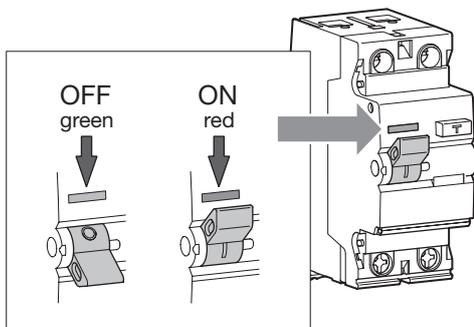
Earth leakage fault indication
