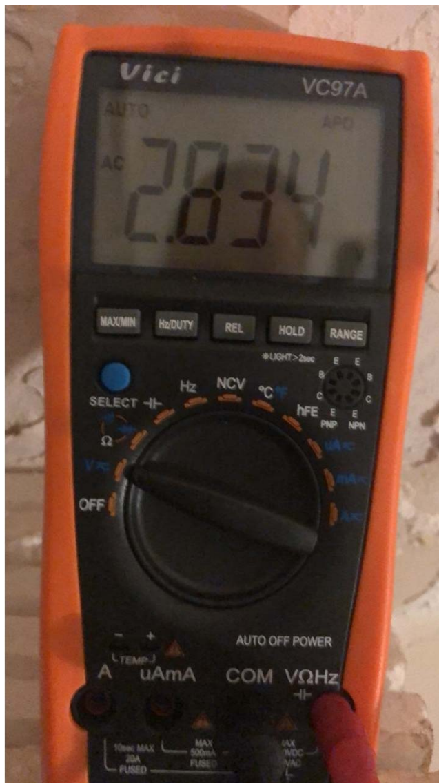
Earth to neutral AC volts in garage
